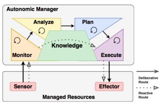
Figure 1. Autonomic Manager in the MAPE-K Architecture [adapted from (IBM, 2005)].
