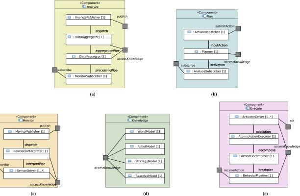
Figure 2. Representation of the internal structures of the Monitor (c), Analyze (a), Plan (b), Execute (e), and Knowledge (d) components.
