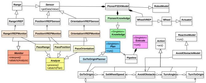
Figure 6. Implementation using the RoCS framework for the Pioneer P3DX. Associations that can be inferred from Figure 3 have been omitted for simplicity.
