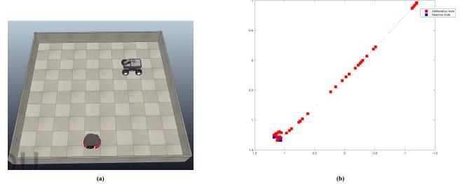
Figure 7. Simulated environment for EXP2 (a) with the two robots R1 and R3 deployed. The robot at the bottom is R1, the disturbing element that is not running the framework. The plot (b) depicts the resulting trajectory and the corresponding active paradigm for the robot that implements the framework. The red/blue trajectory is the R3 trajectory. A video with the resulting simulation can be found at https://youtu.be/2tkBhFGN0Jo.
