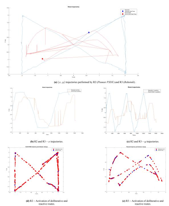
**Figure 9.** EXP3 Results. a) Trajectories (x,y) performed by P3DX with RoCS and Robotnik. (b) X-trajectory performed by both robots. (c) Y-trajectory performed by both robots. (d) P3DX with RoCS behavior execution showing deliberative and reactive routes and behavior switch (squares indicate a change of behavior) (e) Robotnik with RoCS behavior execution showing deliberative and reactive routes and behavior switch (squares indicate a change of behavior).
