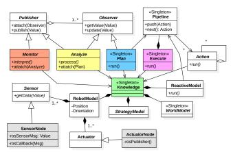
Figure 10. Class Diagram of the RoCS Framework integrated with a ROS environment. The nodes instantiate SensorNode and ActuatorNode objects, allowing RoCS to receive data from subscribed topics and to publish messages, respectively.
