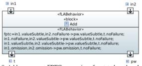
Fig. 8. Add component FPTC expressions for state-based analysis.
