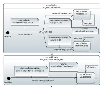
Fig. 7. Electronic Pedal component error models.
