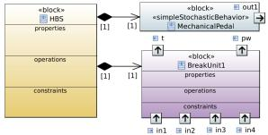
Fig. 2. Excerpt of the HBS block definition diagram in CHESS-ML.
